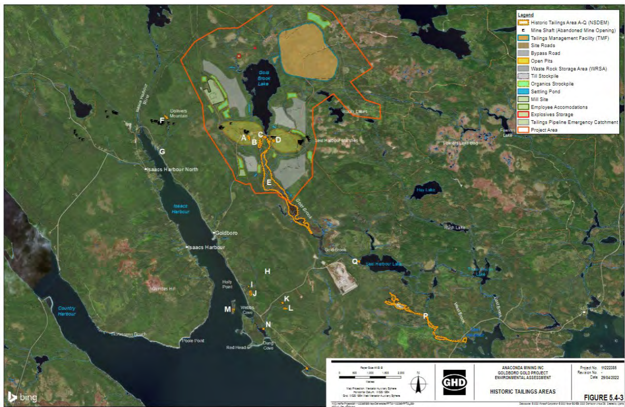
Figure 2. Goldboro Gold Project Infrastructure and Historic Tailings
